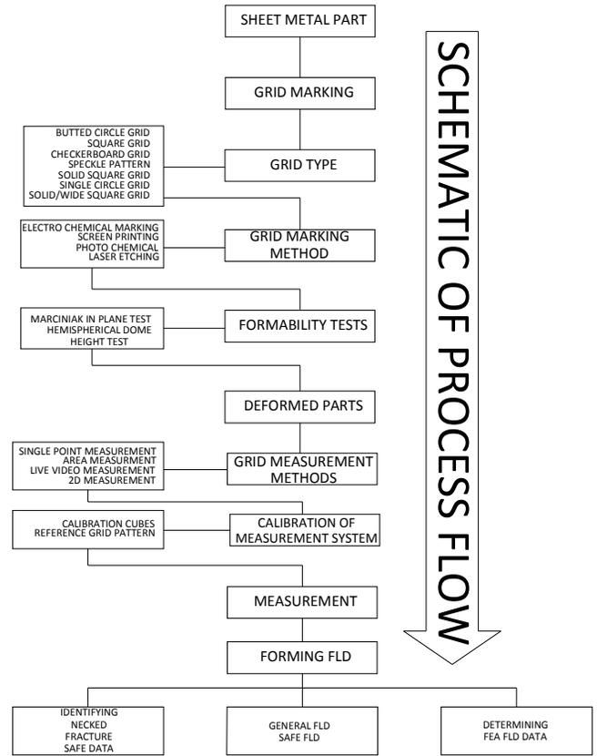
Figure 3: Grid marking and measurement procedures
