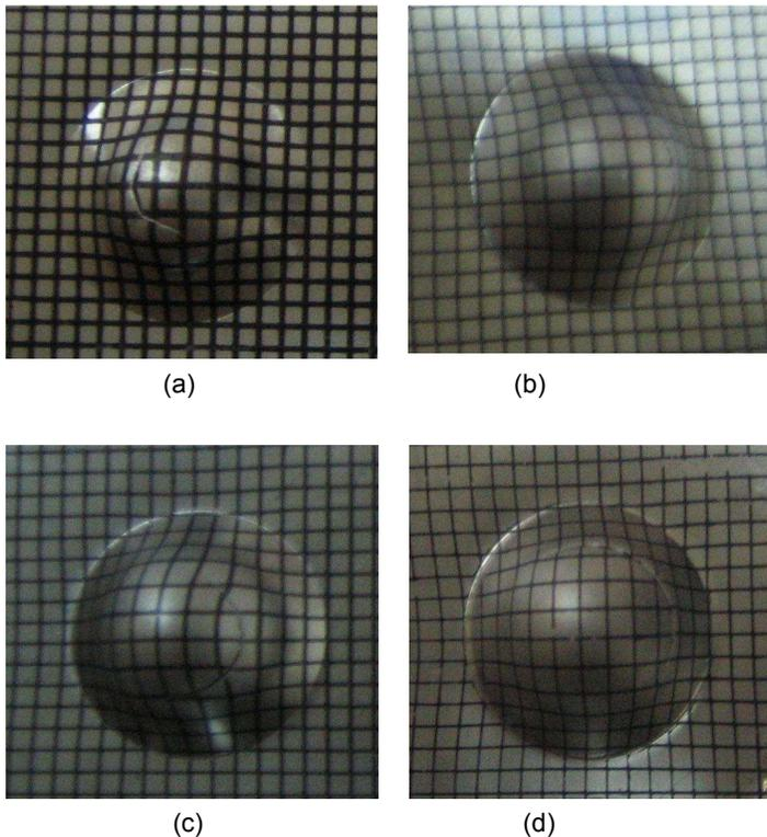
Figure 16: Durability of Serigraphy grid by Erichsen test (a) AA 1050 (b) Titanium (c) DKP steel (d) Stainless steel
