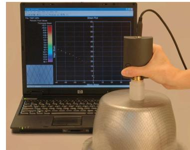
Figure 11: Single point analysis system
