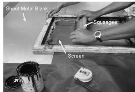
Figure 6: Screen printing process
