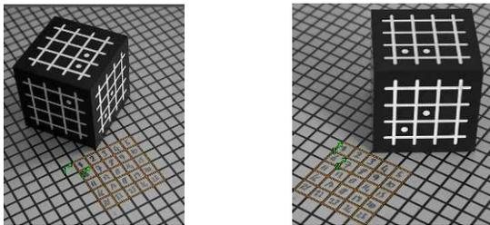
Figure 14: Photographs of 5x5 square grid region taken from two different angles
