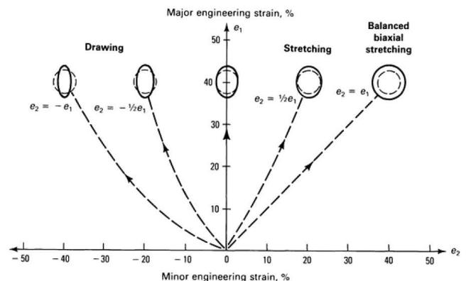
Figure 1: Schematic of several major strain/minor strain combinations in FLD [1]
