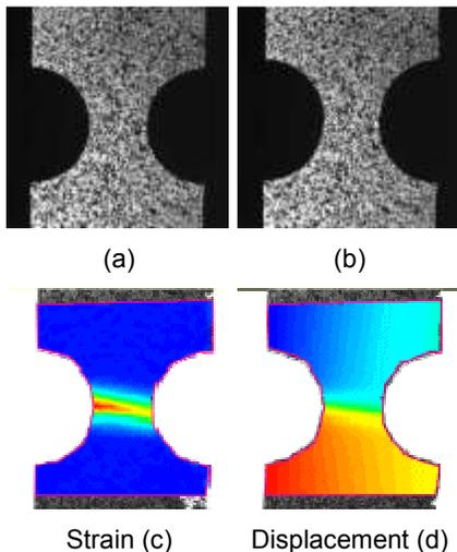
Figure 10: ICASOFT deformation measurement systems.
