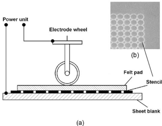
Figure 5: (a) The basic principle of electrochemical etching method [5], (b) example of a stencil
