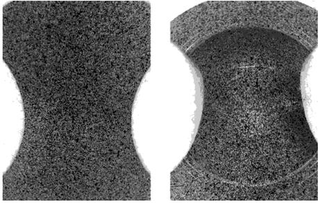
Figure 8: Before and after deformation stochastic pattern
