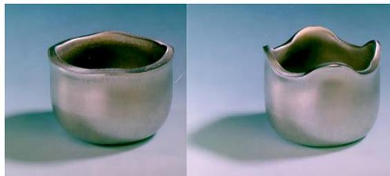
Fig. 1 Two deep drawn cup which shows earing behavior [20]
