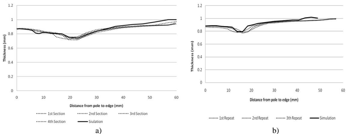
**FIGURE 9.** Geometric comparison of a) 50 mm and b) 200 mm obtained with simulation and 3D scanning
