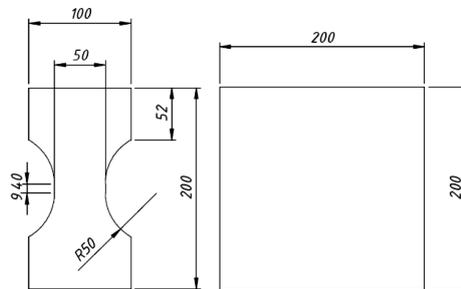
**FIGURE 1.** The specimens used measuring strains on them.
