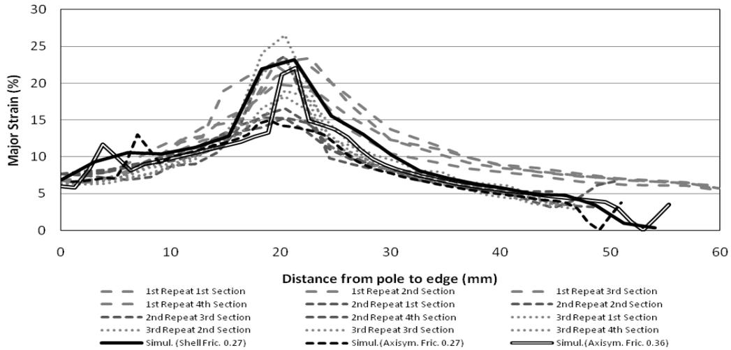
**FIGURE 6.** Comparison of the strain distributions of the measured and simulated 200 mm width part which pass from pole to the edge of the part. Measurements were obtained from three repeated tests. As seen in the figure, the simulation result for shell elements with  $\mu$  of 0.27 and for axisymmetric elements with friction coefficient of 0.36 were well correlated with the test results. As a result both of the element types may be convenient for the simulations.
