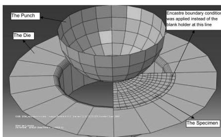
**FIGURE 4.** FEM model of the stretching process
