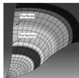
**FIGURE 5.** Major strain distribution and the comparison section of the 200 mm width
