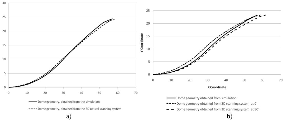
**FIGURE 8.** Geometric comparison of a) 50 mm and b) 200 mm width parts obtained with simulation and 3D scanning
