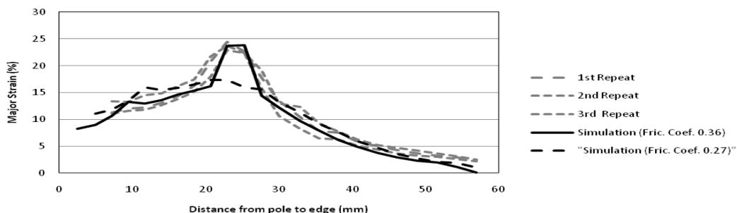
**FIGURE 7.** Comparison of the strain distributions of the measured and simulated 50 mm width part
