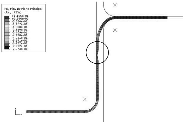
**Figure 4.** The analysis result of using inappropriate parameter values
