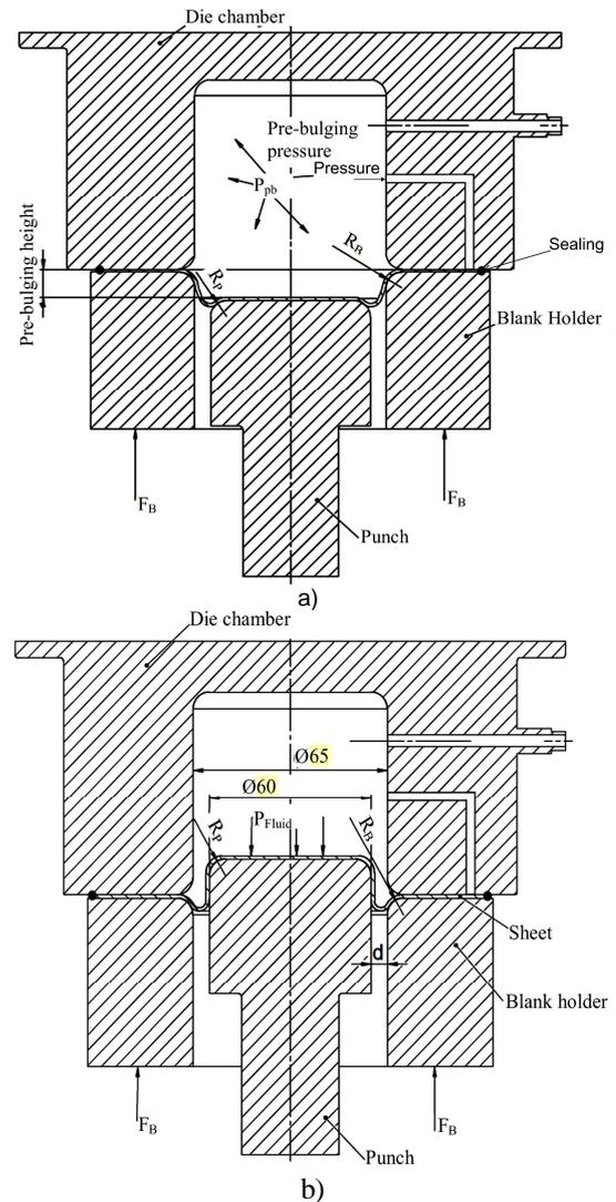
**Figure 1.** The experimental setup of HDD process, a) pre-bulging step, b) forming step
