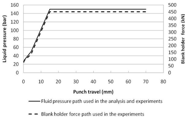
**Figure 5.** Fluid pressures and blank holder force paths used in the analysis and the experiments
