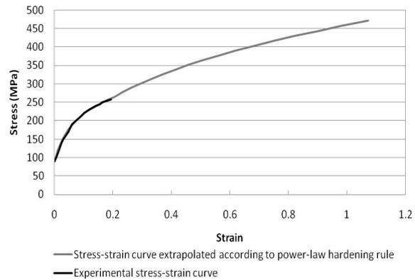
**Figure 3.** True stress-strain curve of the AA 5754-O material (Turkoz et al 2010)
