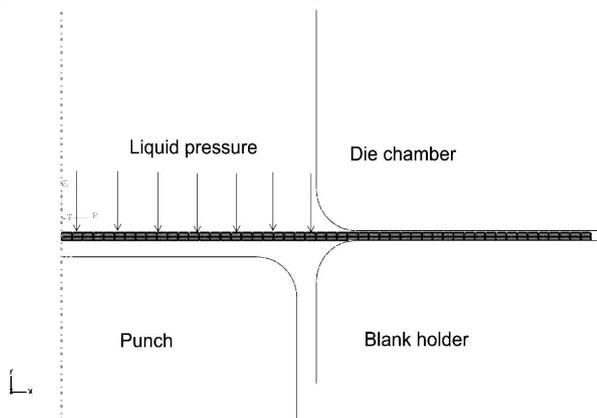
**Figure 2.** The FEM model of the HDD process
