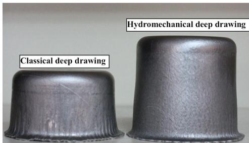
**Figure 9.** The deep drawn cups formed by classical deep drawing and HDD process
