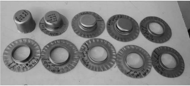
**Figure 8.** Examples of the failed specimens.
