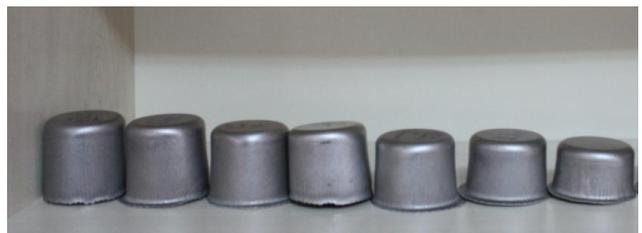
**Figure 7.** The successfully deep drawn cups formed by HDD process
