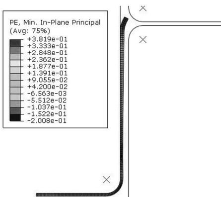
**Figure 6.** The analysis result of successfully formed cup by the HDD process
